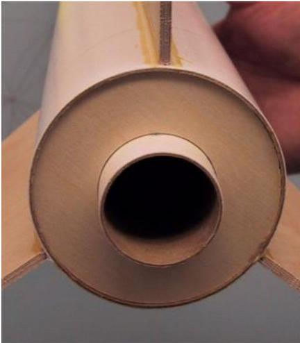
1) The rear ring may fit too tightly if there is any extra glue remaining from the previous steps. Test fit it into the back end of the rocket's main tube, **but be careful. The rear ring may fit so tightly during the test fit, that you may not be able to remove it for gluing.** Sand or scrape the glue residue from the inside back end of the main tube. Or, you may have to sand the outside edge of the ring.
