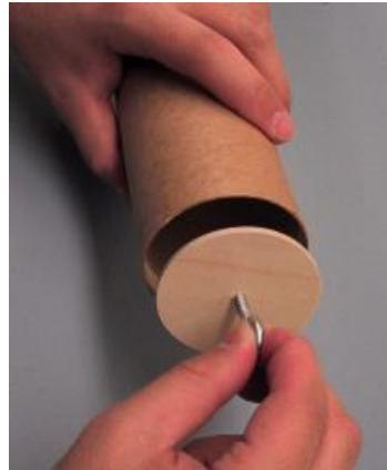
5) Apply a line of glue inside the end of the coupler. Insert the bulkhead ring into end against the glue. Leave about 1/8 of an inch of the coupler showing at the back of the bulkhead ring.
