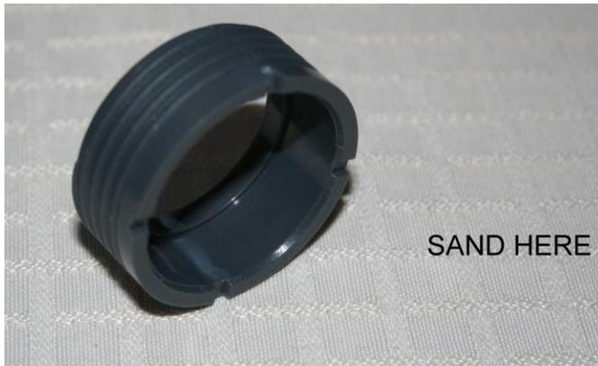
1) Lightly sand the outside of the 29 mm motor mount tube that protrudes from the aft end of the rocket. This will help the glue adhere to the tube.
