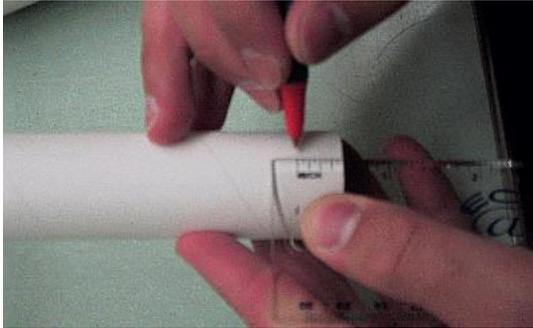
1) Mark a line  $7/16$ " inch from the aft end of the tube (the end without the ring). You will use this mark to know how far to let the motor tube stick out from the end of the rocket.
