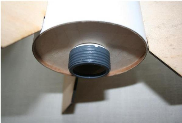
4) Press the motor retainer ring over the motor mount tube until it seats firmly on the motor tube. Wipe away any excess glue. Be careful not to get any glue on the retainer threads or inside the motor tube. The picture to the left shows the retainer ring installed on the LOC IV.
